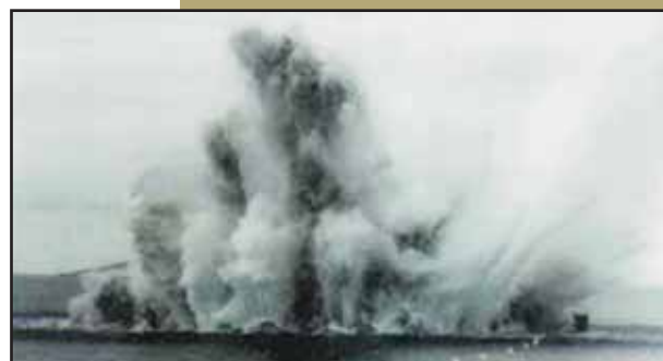
Testing of a sea mine and of marine structures resistance to underwater explosions
