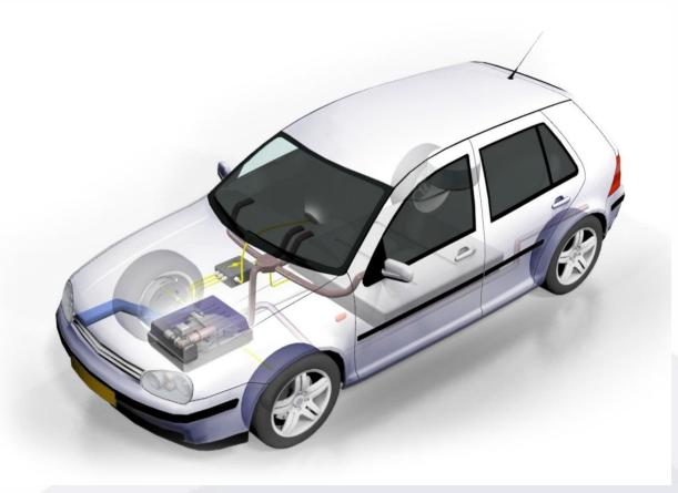
Micro turbine based superior Range Extender technology
