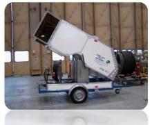
Lately the company produced a new product which prepares washing liquid for cleaning gas paths of CFM 56 and V2500 engines. The GTM 10.1 PRO JET one JUNIOR gas path cleaner equipment is adjusted for providing 19-23 litre/min for CFM engines, and 20-30 litre/min quantity for V2500 engines.
