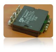
A highly specialized magnetic components designer and manufacturer with many years of experience in the field of custom made conventional and planar transformers for several space and military applications, is proposing the use of a new low profile transformer solution to be used in several military medium power applications where high performance and low profile and weight are a necessity. The proposed project includes also potential customization of the planar
