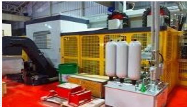
TREVISAN DS600 AT Coimbatore Facility TV-1 : SWING DIA OF CHUCK in mm: 1000 X 1000 Twin Pallet
