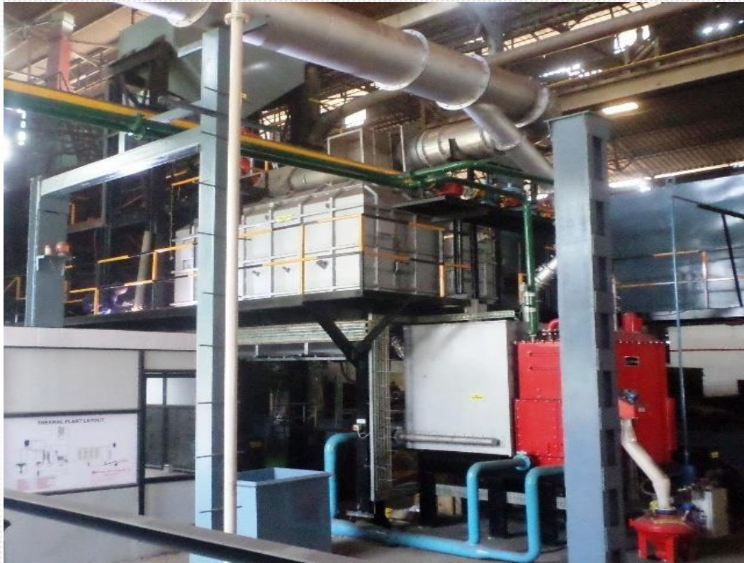
Thermal Sand Reclamation Plant from OMEGA, 3 Ton/hour
