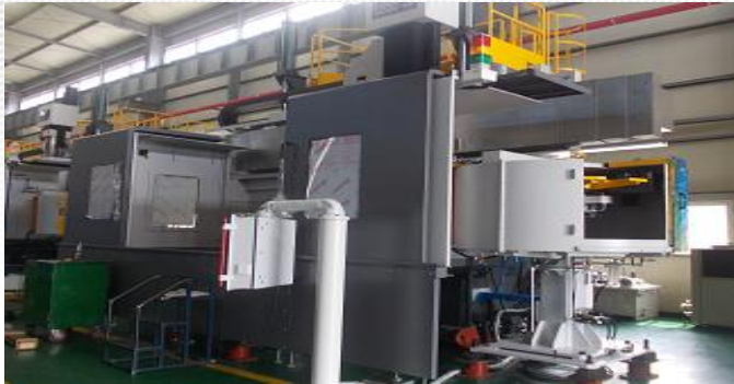
CNC - VERTICAL TURNING LATHE WITH ATC VTL-5 : HNK NT 20/25, SWING-2500mm, HEIGHT-1800mm, LOAD-12MT CONTROL: FANUC 31iA
