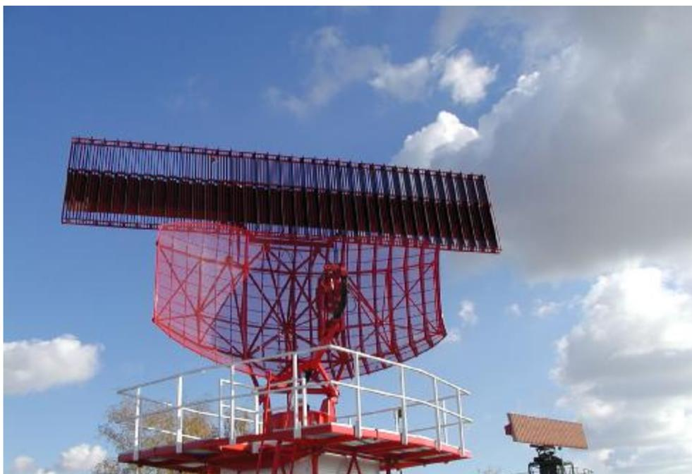
*RL-2000 is latest generation of ELDIS primary surveillance radars for Terminal Approach Control Application. The RL-2000 design is benefiting from the long time experience on several civilian and military radar types. The radar meets or exceeds ICAO and EUROCONTROL recommendations and standards. The RL-2000 features fully solid-state highly modular configuration, fail-safe system and low life cycle cost.*
