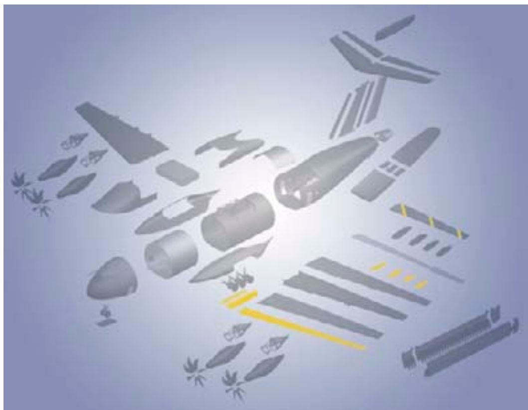
A400M - work-share for Belgian companies: landing gear doors, leading edges, flap supports and flap skins.
