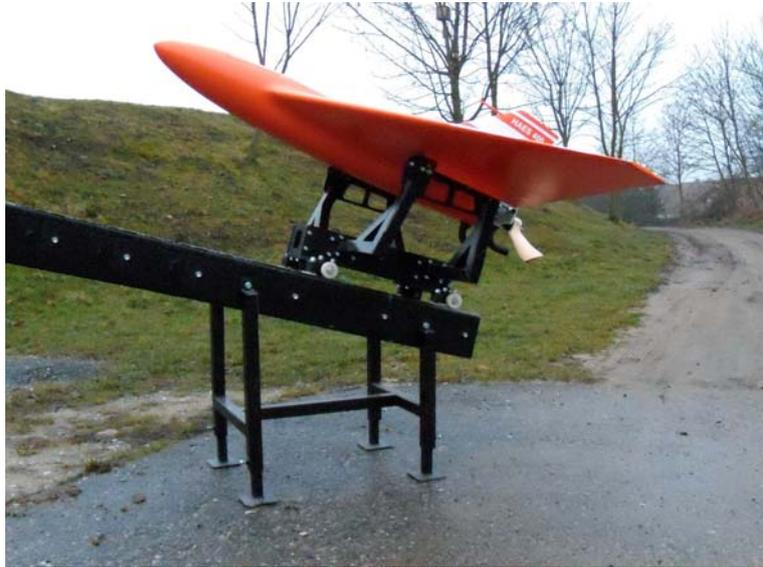
The drone is launched from a rail system. The drone can be recovered by a parachute recovery system. Recovered targets are repaired, tested and reused. The HAES 400 can carry a full range of current target payloads which include infrared and radar enhancements and a chaff/flare dispenser set.
