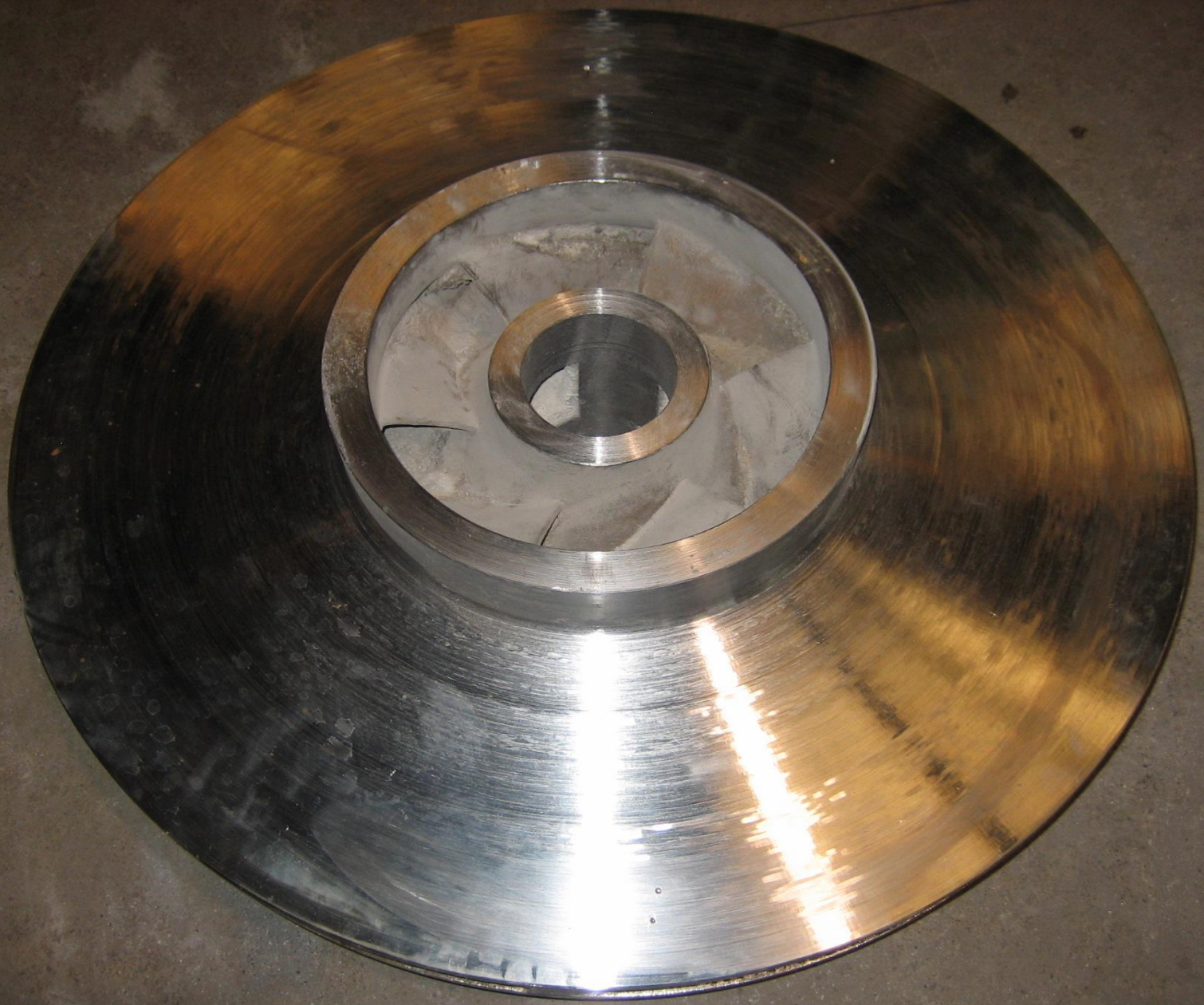
164 Kg Impeller in semi-finished condition
