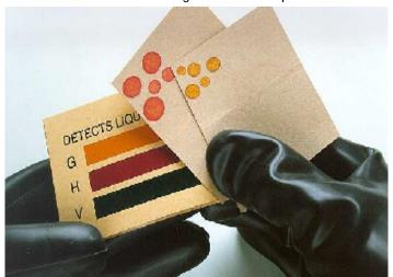
chemical warfare agents G, V and H in a liquid form. Drop of chemical agent creates immediately colour spot on the paper. According to the colour is possible to determine groups of the G, V, and H agents within 30 seconds.
