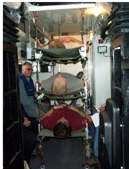
Shock and vibration damped stretcher rack on board the Norwegian Coastal Ranger SB90N Battle Boats
