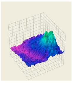
First test images of living cells in nanometer depth resolution using confocal probe. Upper image: depth profile in false colours, lower left image intensity profile in false colours, lower right 3D image showing that elevated part of the cell have lower reflectivity –
