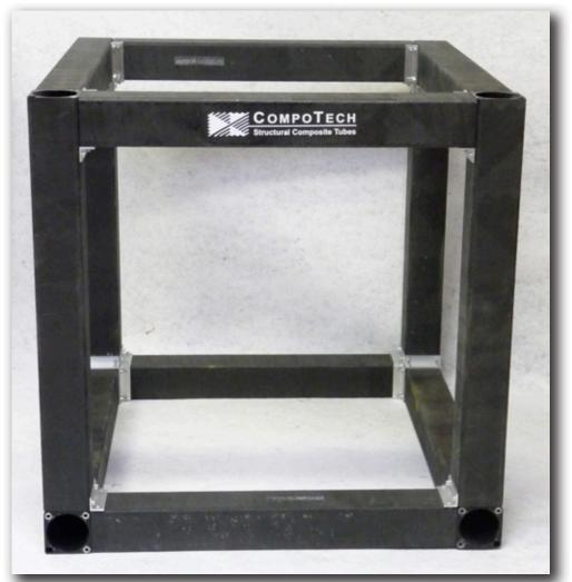
This is achieved by using a combination of high strength and high modulus carbon fibres laid in a matrix of epoxy resin with carbon nano particles. These tubes also have very good dynamic vibration characteristics which are also important for the accuracy of the optical instruments.
