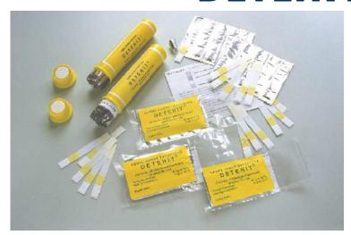
The detector strip DETEHIT® was designed for detection of nerve agents in air, water, food and on the surface. The detection strip can determine dangerous concentrations of nerve agents in the air (within 2-3 minutes), if it is possible to remove the gas mask (5-15 minutes) or whether food or water are acceptable for intake (15-30 minutes).
