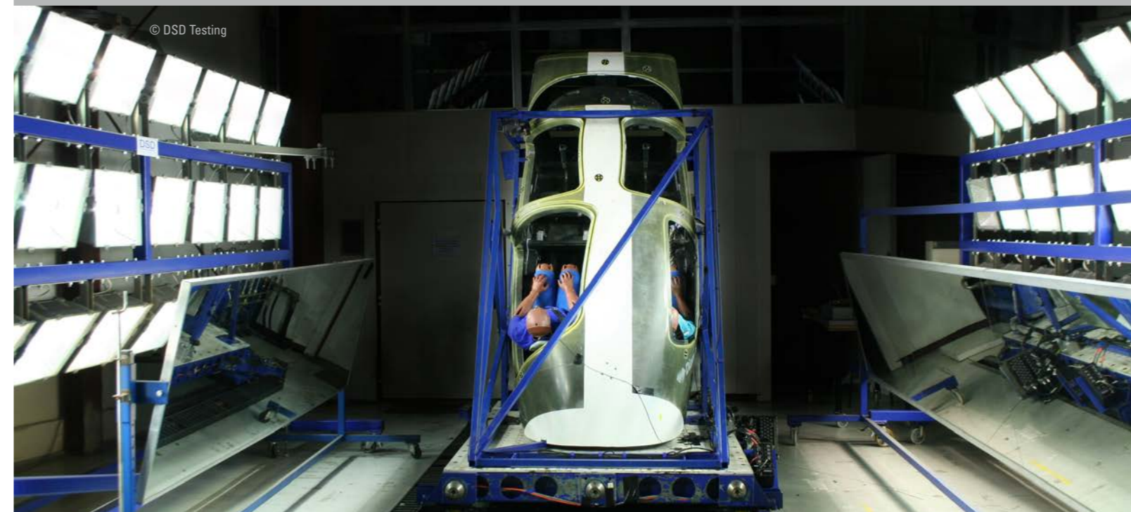
Full scale impact testing with instrumented Crash Test Dummies (image above) and unlimited airframe lifetime (image below)
