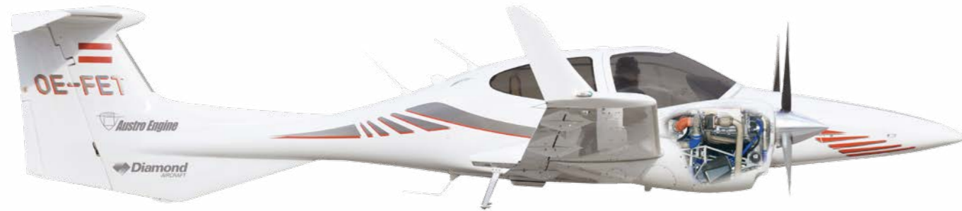
Diamond Aircraft DA42-VI powered by the AE300 Heavy Fuel Engine
