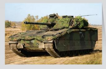
**CV90** | Place of origin: Sweden, In service since: 1993, Weight: 23-35 tonnes, Length: 6.55 meters, Width: 3.1 meters, Height: 2.7 meters, Speed: 70 km/h, Operational range: 320 km, Transmission: Automatic, Engine: 550-810 hp, Crew: 3 (commander, gunner, driver) 6 or 8 troopers.
