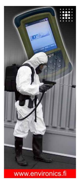
The ID100 is the first truly portable FTIR gas analyzer in the world. The lightweight analyzer module is located in durable Teflon coated backpack. The ID100 analyzer houses a Fourier Transform Infrared (FTIR) spectrometer, Rhodium-Gold coated sample cell and signal processing electronics. The sample gas is extracted into the sample cell with a pistol-type probe. Hence no sample preparation is needed.
