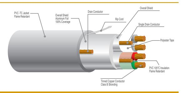
Size 16 AWG Nominal Insulation Thickness: 0,42 mm
