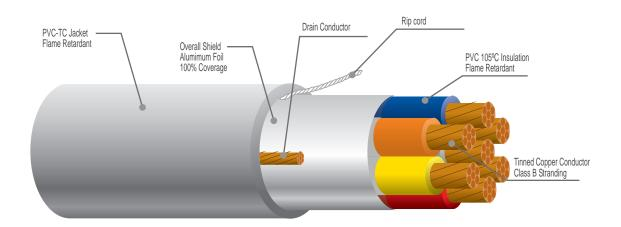
Size 16 AWG Nominal Insulation Thickness: 0,42 mm
