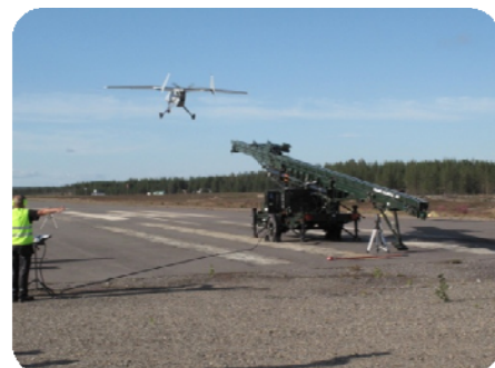
The SELEX Galileo Falco being launched off the Robonic MC2555LLR at the RATUFC range
