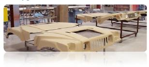
A leading company in the development manufacturing of composite products for ballistic protection and structural composite applications is proposing the development of a new all-composite cabin for future or existing wheeled and tracked military
