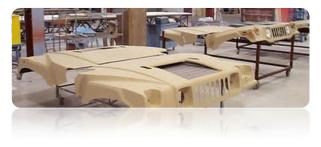
A leading company in the development and manufacturing of composite products for ballistic protection and structural composite applications is proposing the development of a new all-composite cabin for future or existing wheeled and tracked military
