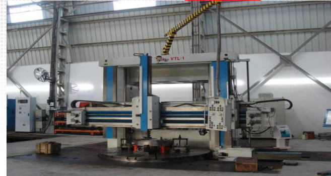
VERTICAL TURNING LATHE VTL-1 : TITAN SC 27, SWING-2630mm, HEIGHT-1900mm, DRO, PLC, LOAD-12MT
