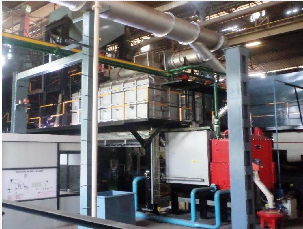
Thermal Sand Reclamation Plant from OMEGA, 3 Ton/hour
