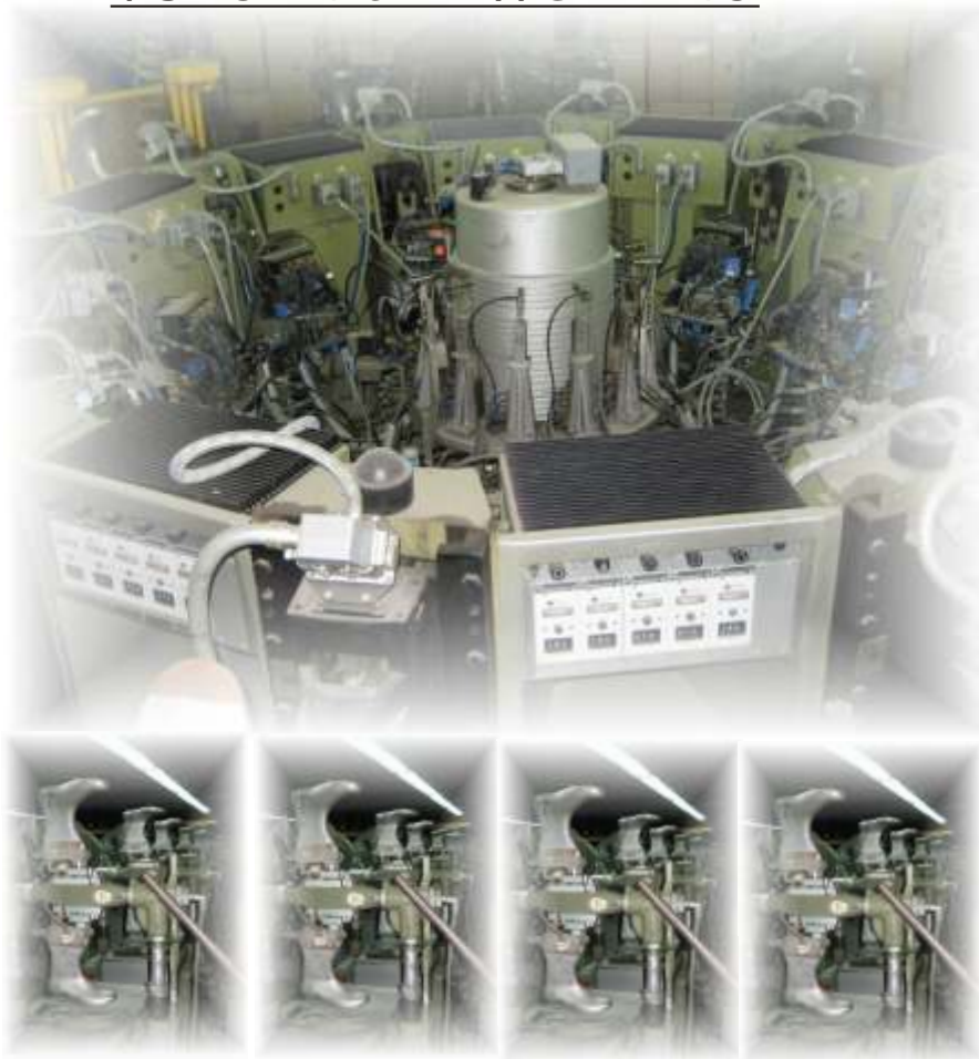
INJECTOR MACHINE FOR MAKING RUBBER SOLES
