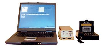
The RCDS<sup>®</sup> consists of computer based Master Crypto Management (MCM) system which is operating system independent and normally runs on a laptop. In its basic configuration, to small rugged boxes are required; one designated as the Master Crypto Unit (MCU) which is normally co-located with the MCM and one designated as the Slave Crypto Unit (SCU), which is normally located at the remote site. The MCU and SCU are connected by an IP secure VPN, i.e in-country Digital Data Network (DDN).
