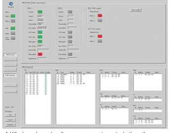
A Windows-based radio management, controls the other system modules from a pair of redundantly connected computers. A firewall prevents and reports illegal commands.
