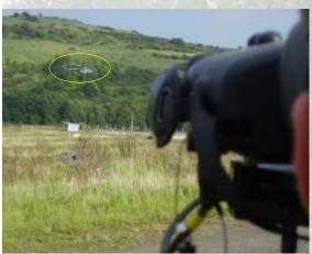
From the technical point of view, the air observer configuration comprises a tripod, a goniometer with connected sensors, a rugged portable computer that communicates with the command & control post by means of a radio or wire. ReTOB operates by one operator only.
