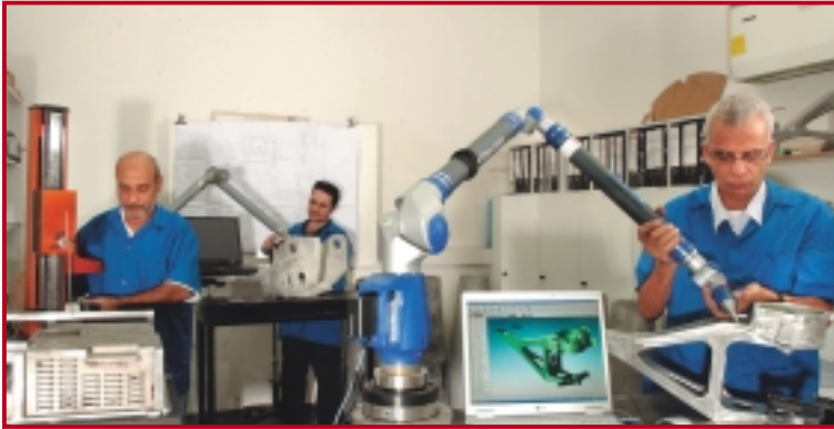
Castings and patterns are measured by two layouts of digital Faro Arm Measuring Machines, using compare to CAD inspection system.
