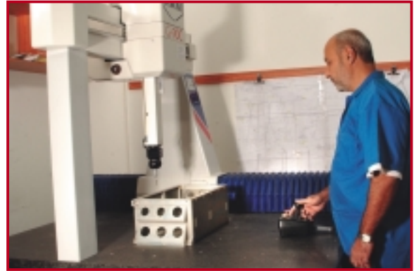
Machined parts are inspected using L.K.'s CNC Coordinate Measuring Machine.
