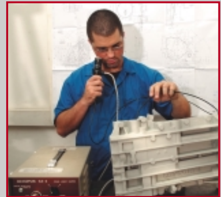
Boroscopic inspection of long and narrow core passages.
