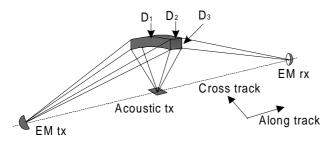
Figure 1. The electromagnetic common volume is illuminated by acoustic energy. Transmitting the proper acoustic frequency generates a narrow volume of Bragg scattering. The electromagnetic energy scattered from this volume is shifted by the acoustic frequency.
