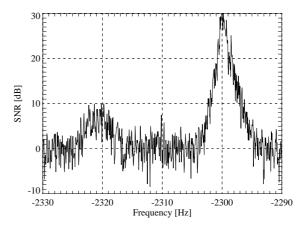
Figure 10. Power spectra of a received EM signal. Wind during measurement: 4.0 m/s cross track and -9.0 m/s along track.
