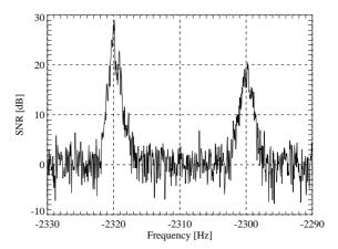
Figure 9. Power spectra of a received EM signal Wind during measurement: -1.3 m/s cross track and -5.5 m/s along track.
