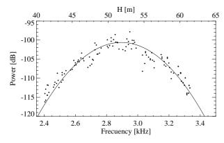
Figure 8. Experimental data (dots) and the theoretical curve for energy distribution and scattering angle dependency. Each point of data represents 6 seconds integration time. The measured points match the theoretical curve well.
