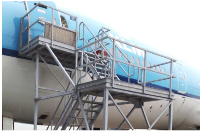
Access Stair for Maintenance
