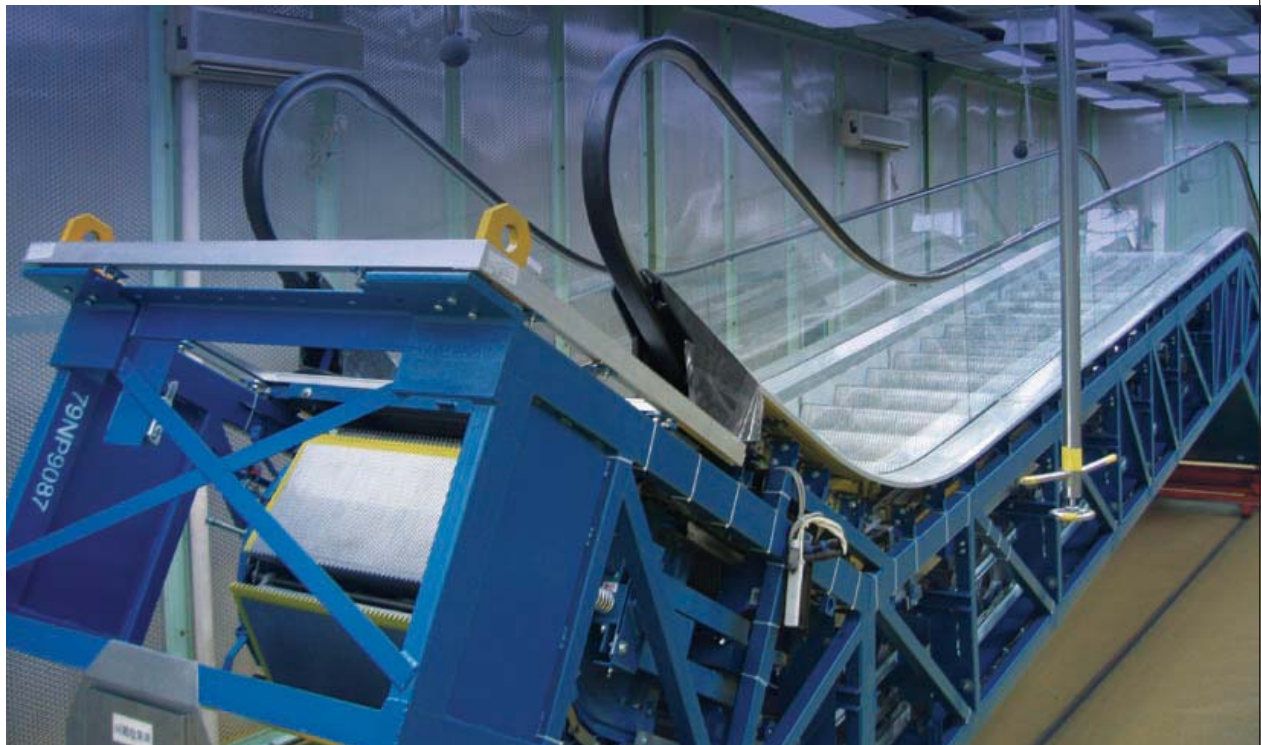
Final Assembly and Tests being conducted (FATS)
