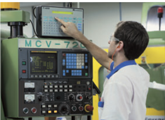
All machines and processes have terminals for DNC and production shop floor data collection.
