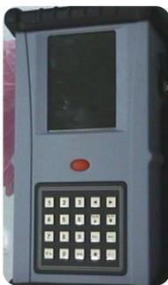
A leading company in the design and production of various engine component test stands and health monitoring systems is proposing the adaptation (including necessary hardware and software tools) of an existing Data Retrieval Unit specially designed for F100-PW-220/229, F110-GE-129 and T700-GE-701C type of engines, in order to perform the required health monitoring and testing procedures for an alternative modern civil or military jet engine defined by any likewise interested Prime.
