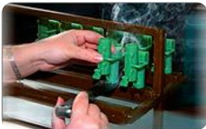
A company specialized in the manufacture of precision castings steel and aluminum parts using the Lost Wax Process for the defense and industrial sectors, is proposing, in the frame of an offset program, the collaboration with Aerospace and Defense (A&D) primes or lower tier companies for the provision of Rapid Prototyping services for new steel and Aluminum casting designs for specific Aerospace applications.
