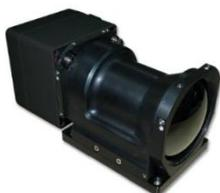
**Arbel™** - Dual FOV uncooled thermal OEM Camera for surveillance and weapon stations, available in a variety of forms, including 384X288, 640X480 and high sensitivity 640X480 resolutions. Field proven - thousands of units installed.
