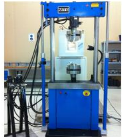
MTS 100kN Mechanical Test Bench for Both Static and Dynamic
