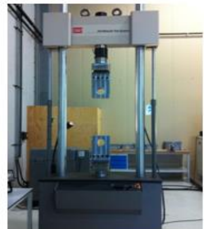
MTS 500kN Mechanical Test Bench for Both Static and Dynamic
