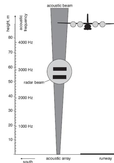
Bi-static radar setup provides an advantage over other radio-acoustic systems and makes it possible to measure in several altitudes simultaneously with fine resolution in space and time.
