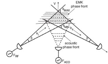
Based on Bragg wavenumber matching between electromagnetic and acoustic waves.
