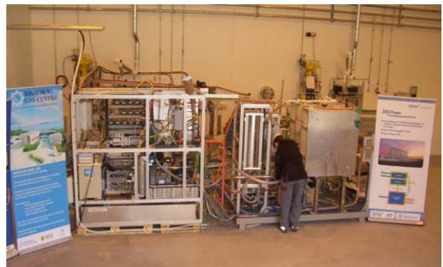
Figure 3. The ZEG-power plant, combined electricity and hydrogen production with CCS.
