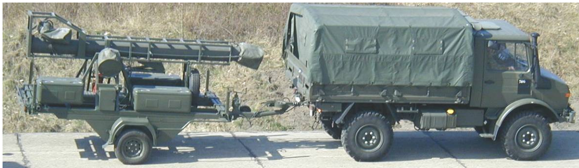
30m mast on trailer, for LOS system (headload 50kg)
