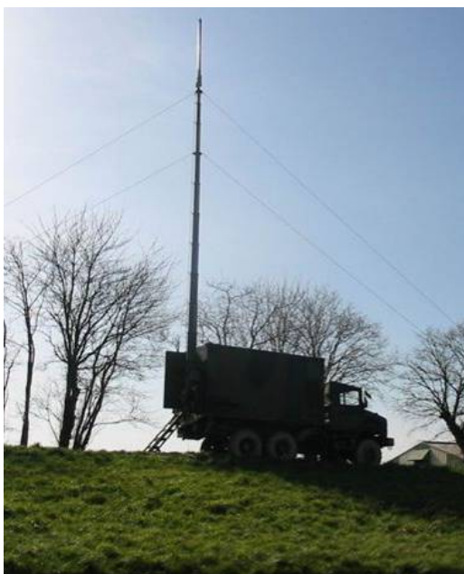
12m mast on Shelter for L16 links
