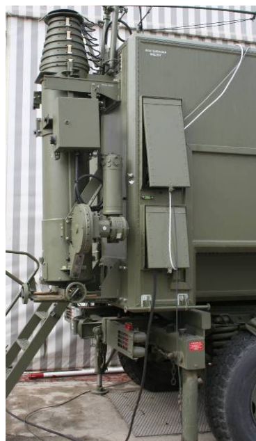
8m mast supporting 120kg (EW system)
