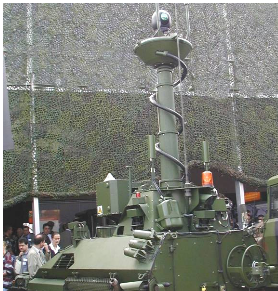
5m mast integrated inside armoured vehicle (headload 170kg)
