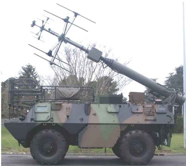
16m mast on LAV, for E.W. system (headload 300kg)
