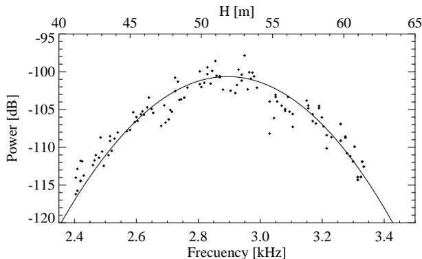
Figure 8. Experimental data (dots) and the theoretical curve for energy distribution and scattering angle dependency. Each point of data represents 6 seconds integration time. The measured points match the theoretical curve well.
