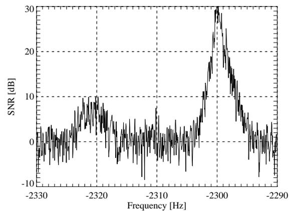
Figure 10. Power spectra of a received EM signal. Wind during measurement:  $4.0$  m/s cross track and  $-9.0$  m/s along track.
