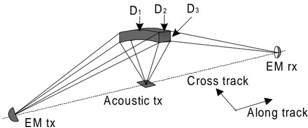
Figure 1. The electromagnetic common volume is illuminated by acoustic energy. Transmitting the proper acoustic frequency generates a narrow volume of Bragg scattering. The electromagnetic energy scattered from this volume is shifted by the acoustic frequency.
