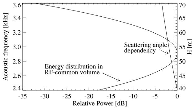
Figure 7. The scattering angle dependency and the EM common volume Gaussian energy distribution plotted versus the height and matching frequency (for zero degrees air temperature).
