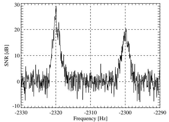
Figure 9. Power spectra of a received EM signal Wind during measurement:  $-1.3$  m/s cross track and  $-5.5$  m/s along track.
